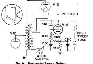
Fig. 6. Horizontal Sweep Output
