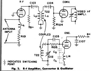
The windings are self-tuned by the distributed and tube capacities to provide optimum gain. On channels No. 1 and No. 2 the transformer is triple tuned to prevent the image frequencies of the 88-108 mc FM band from interfering with these two channels. The triode converter is one section of a Type 7F8 dual triode, V2A. Bias for this tube is provided by the oscillator voltage appearing in the grid of V2A causing grid rectification charging the grid resistorcondenser combination, R104 and C104.
